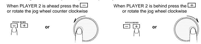
The pitch changes automatically while the  $\pm$  or  $\Box$  button is being pressed or the jog wheel is rotated. The faster you rotate the wheel the more you change. Releasing the button or wheel results in a return to the original pitch. (So the BPM's are once again the same.)
